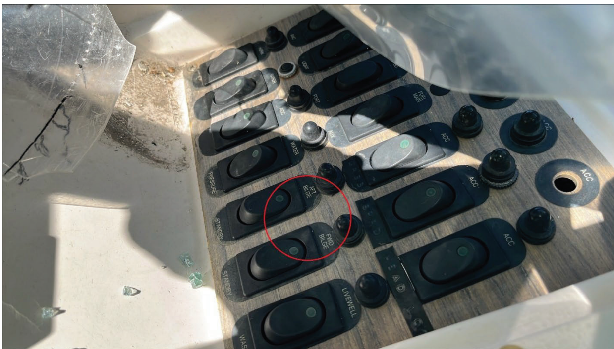
Figure 3: Photo of the main console taken by USCG. Showing both bilge pumps were in the on position.
